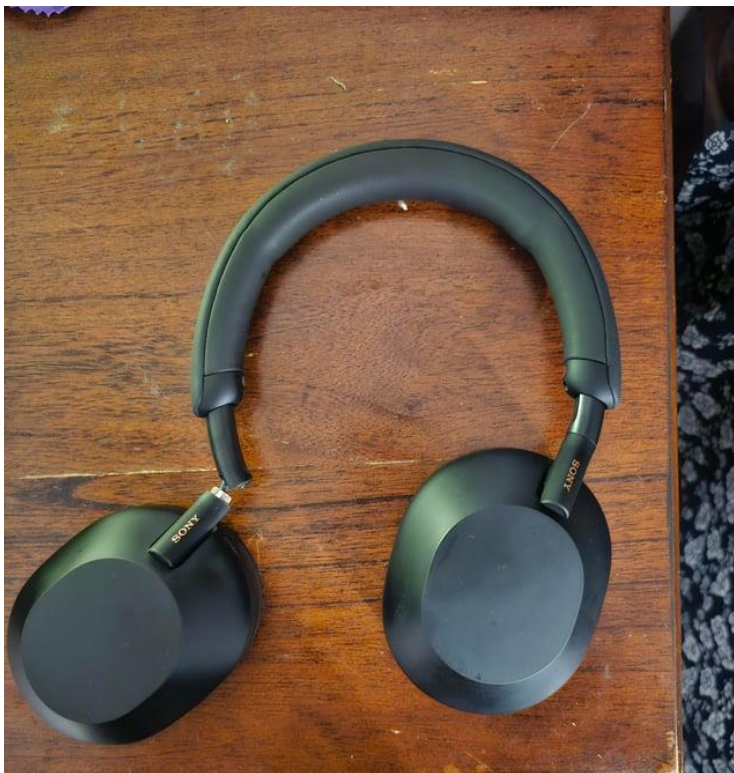
Figure 1: Fully Detached Swiveling Hinge Due to Defect. 1
